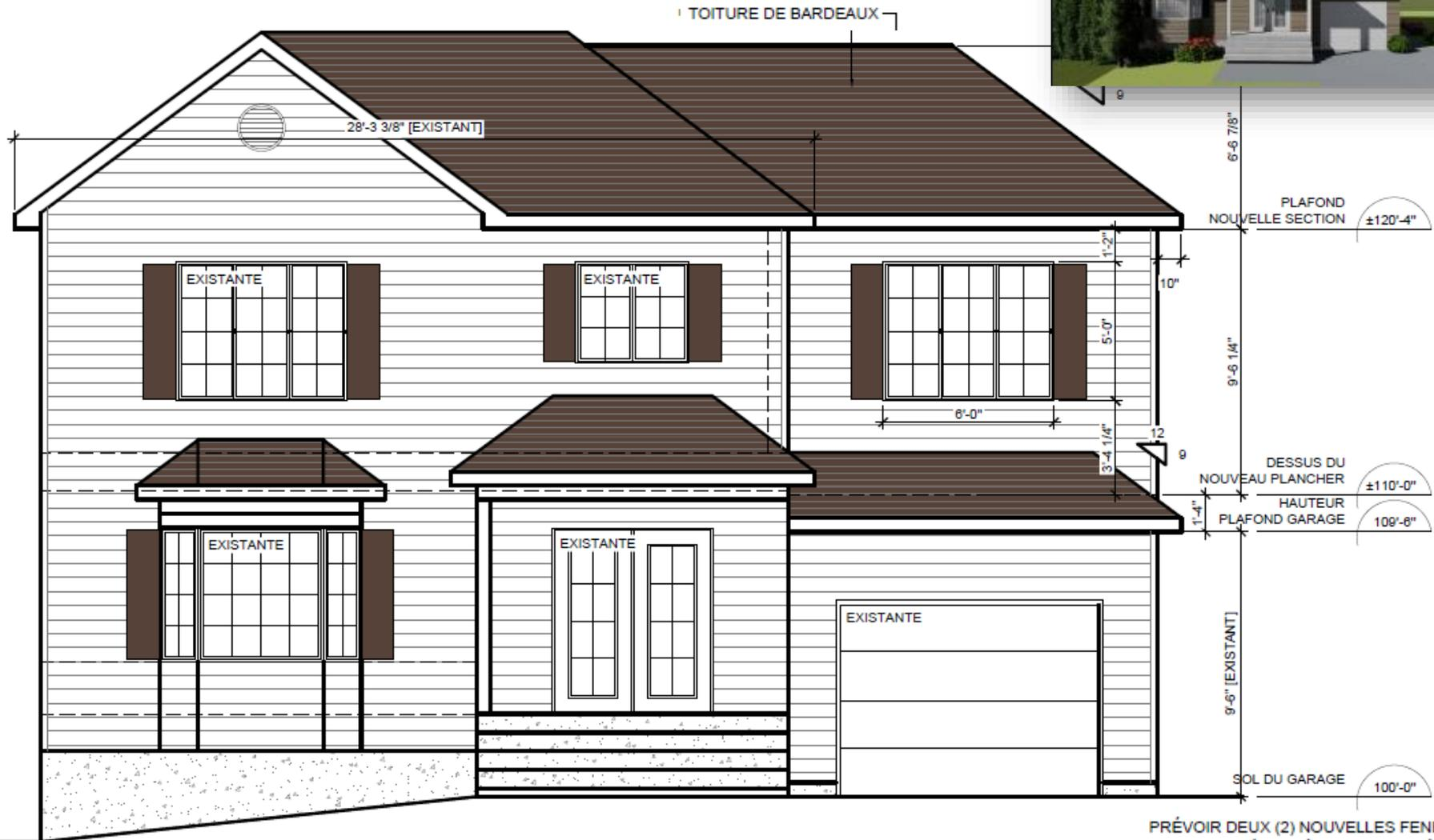
ÉLÉVATION - FAÇADE - AJOUT D'ÉTAGE AU-DESSUS DU GARAGE
